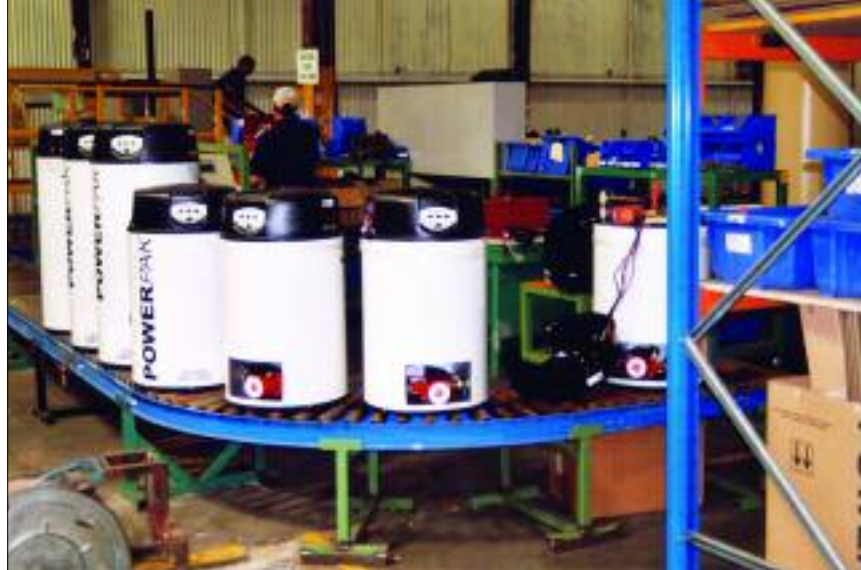
Final installation of the Australian Powerpaks: with these compact units the sun can be connected to existing tanks.
